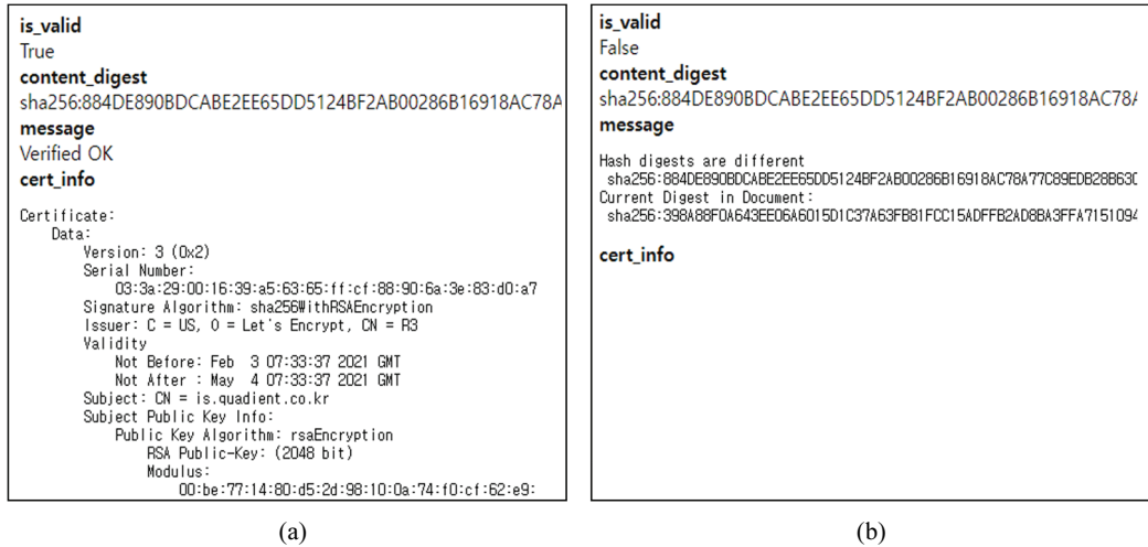
Fig. 13. The verification results: (a) the valid Document HTML and (b) the invalid Document HTML.
